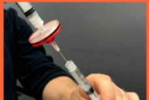
Attach primed filter to barrel and add blunt tip to other end of the filter
